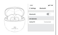
If the pairing fails, put the earbuds into the charging case, and then try the steps above again, the earbuds will automatically shut down when there is no devices to connect in 5 minutes.
